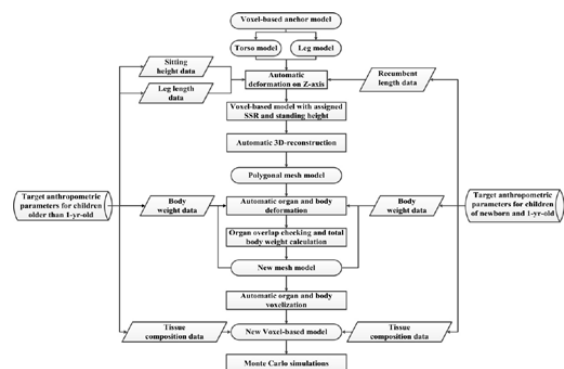
Figure 1. Flowchart of phantom remodeling for Monte Carlo simulations
